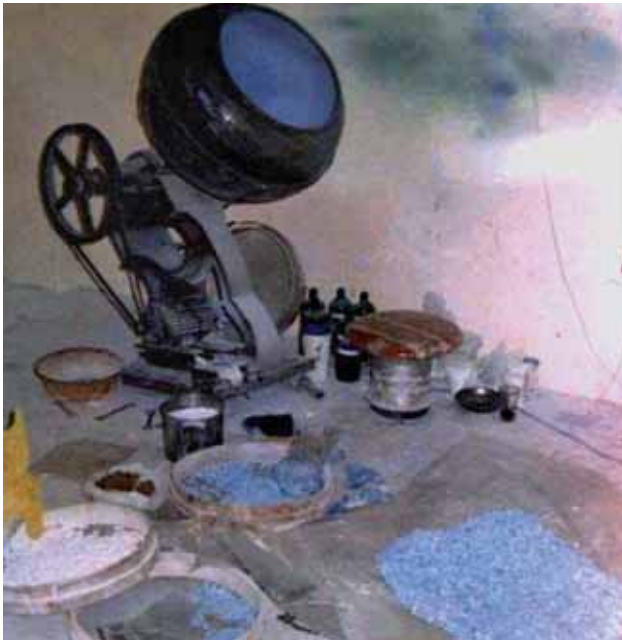
Figure 4 – Counterfeit drug manufacturing device from Egypt.
