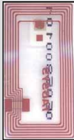
Figure 7 – The V-tag program in the USA: a unique tag is placed on each bottle of Viagra® during production and a web-based system permits pharmacist to verify authenticity.
